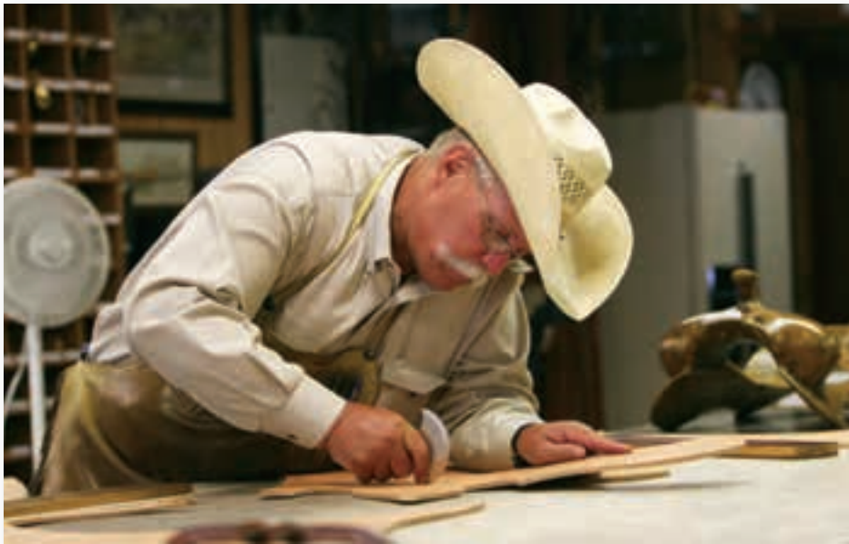
Wade makes a series of leather cuts. He uses Hermann Oak leather exclusively, preferring it for its strength and longevity
