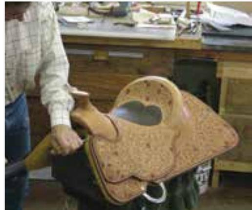
The skirts are placed back on to stay. The skirt edges have been oiled a bit, then hot-waxed. I'm on the downhill side of the project at this point. Note how the bottom line of the front jockey is parallel with the bottom line of the skirt. If these are not parallel, even a novice can pick up that something's amiss.
