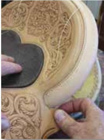
The cantle binding has been sewn by hand. One of the marks of an accomplished saddler is how parts and pieces fit together – for example, working hard for a nice, clean fit of the seat leather as it draws around the Cheyenne roll. Technically clean work will give the whole project an attractive aesthetic.
