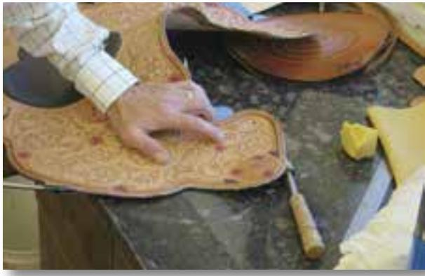
During a 2009 visit to France, I learned to hot-wax edges of leather. A specially designed heated iron locates beeswax into the pores of the leather edges. I've oiled the edges of the seat so the wax will co-mingle with the neatsfoot oil, creating a durable, attractive edge.
