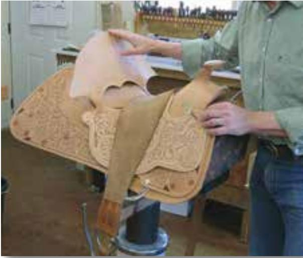
The seat has been carved and colored. I've cut out the hole where the inlaid cushion seat is to be installed. The drawdown strap is used often in this process to build shape into the seat leather and to hold it in place. You can see the smaller medallion on the front jockey, above the larger one on the skirt.
