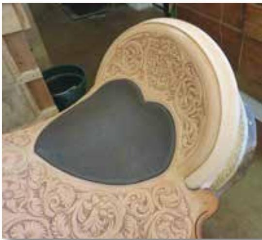
The cantle binding has been glued on and is ready to sew. This binding has a rolled front edge I put on all my museum-grade saddles. The edge of the binding is carefully skived down to a feather edge, then folded and glued in order to create a clean edge at the stitch line.
