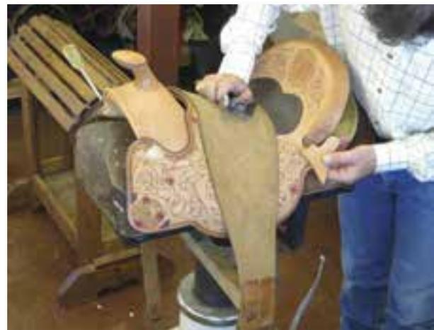
The cantle dish has been carved and the seat is glued in to stay. Here, I'm cutting filler pieces for a narrow Cheyenne roll.
