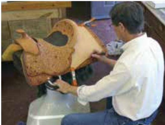
Now the back jockeys are cut out. As noted earlier, the bottom line of the back jockey needs to correspond with the bottom line of the front jockey. We're after compatible architectural lines.
