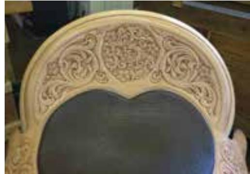
The cantle binding has been sewn. Note the nice, even reveal of the Cheyenne roll as it travels from one side to the other. Color has yet to be added to the decoration. The floral carving design must respect the shape of the cantle. Here we see the largest element (the medallion) in the center, with a graduating sequence of smaller elements as the area tapers off to the corners.
