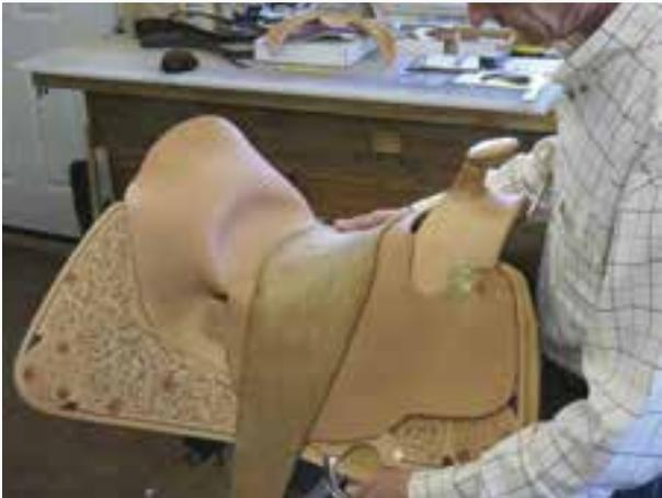
The cuts have been made on the saddle seat. The seat leather is then placed back on the tree in order to allow it to dry in preparation for carving. You can see how the front cut on the front jockey has followed the front line of the skirt.
