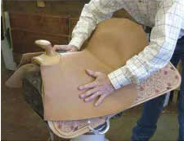
The rigging hardware has been installed using rivets with Scott Hardy silver heads. I'm ready to cut out the seat leather. It's important to have the skirts on during this process because the skirts are the foundation the rest of the parts are cut and built upon. The skirts are the base form that needs to be respected in all the other cuts of the saddle. The leather is very wet and moldable at this point.
